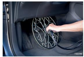
NOTE: When using the hand-held array without the reflective plate (as for acoustic holography measurements) noise will reflect off of the tablet. Remove the tablet from the holder to prevent the detection of such sounds.
