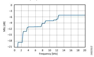
The array is optimized for both acoustic holography and beamforming measurements, with a patented numerical method to optimize performance for the frequency range and number of microphones. See Fig. 3 for the dynamic range, or maximum side lobe (MSL) level, of the array. For more information consult technical review, BV 0056.
